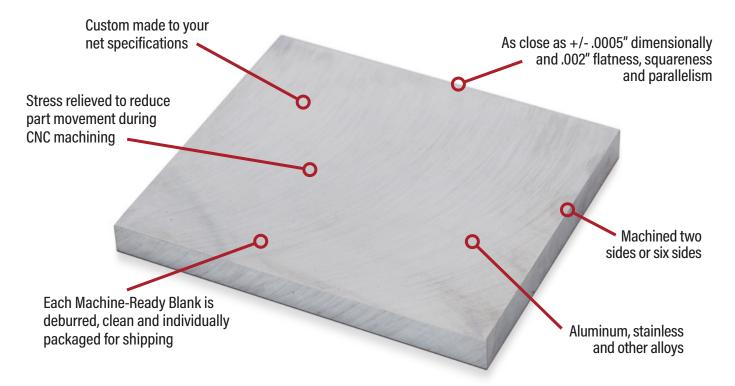
Machine-Ready Blanks from TCI Precision Metals arrive at your shop ready for finish machining. No sawing, squaring, grinding, or other outside services are necessary. Precision blanks are made square, flat, and parallel to as close as +/-.0005" dimensionally and +/-.002" flatness and can be ordered in quantities from one to thousands, with quick turn-around.
